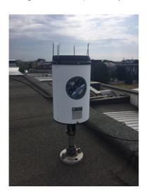
The Thies CLIMA laser disdrometer, installed on the rooftop of Building 20 of DEIB, provides detailed information on hydrometeors by measuring their particles size, their falling velocity and their state (liquid drops, snow flakes, hail particles, ...). Results are output with 1-minute integration time and they are of key importance for the in-depth investigation of the effects of precipitation on EM waves.
